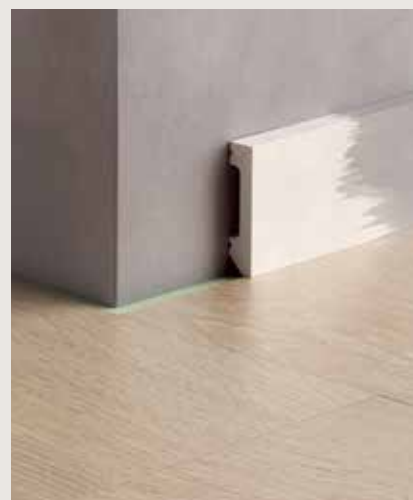
PAINTABLE WATERPROOF MEDIUM SKIRTING 2400 × 13 × 58 mm Paintable, or can be left white. Use the Foamstrip and Aqua Sealant to obtain a watertight finish. Core: polystyrene.
