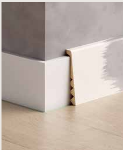
PAINTABLE COVER SKIRTING 2400 × 129 × 16 mm For easy and fast renovation. Covers existing skirting. Paintable, or can be left white. Core: MDF.
